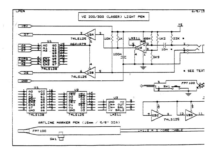
A LIGHT PEN IS AN INPUT DEVICE BETWEEN A COMPUTER AND ITS MONITOR SCREEN AND NEEDS A PROGRAM OR ROUTINE TO CONTROL IT, JUST LIKE A JOYSTICK. ON THE VZ IT'S NOT VERY ACCURATE AND MONITOR SCREEN CONTRAST AND BRIGHTNESS PLAY A BIG PART IN ITS OPERATION.
